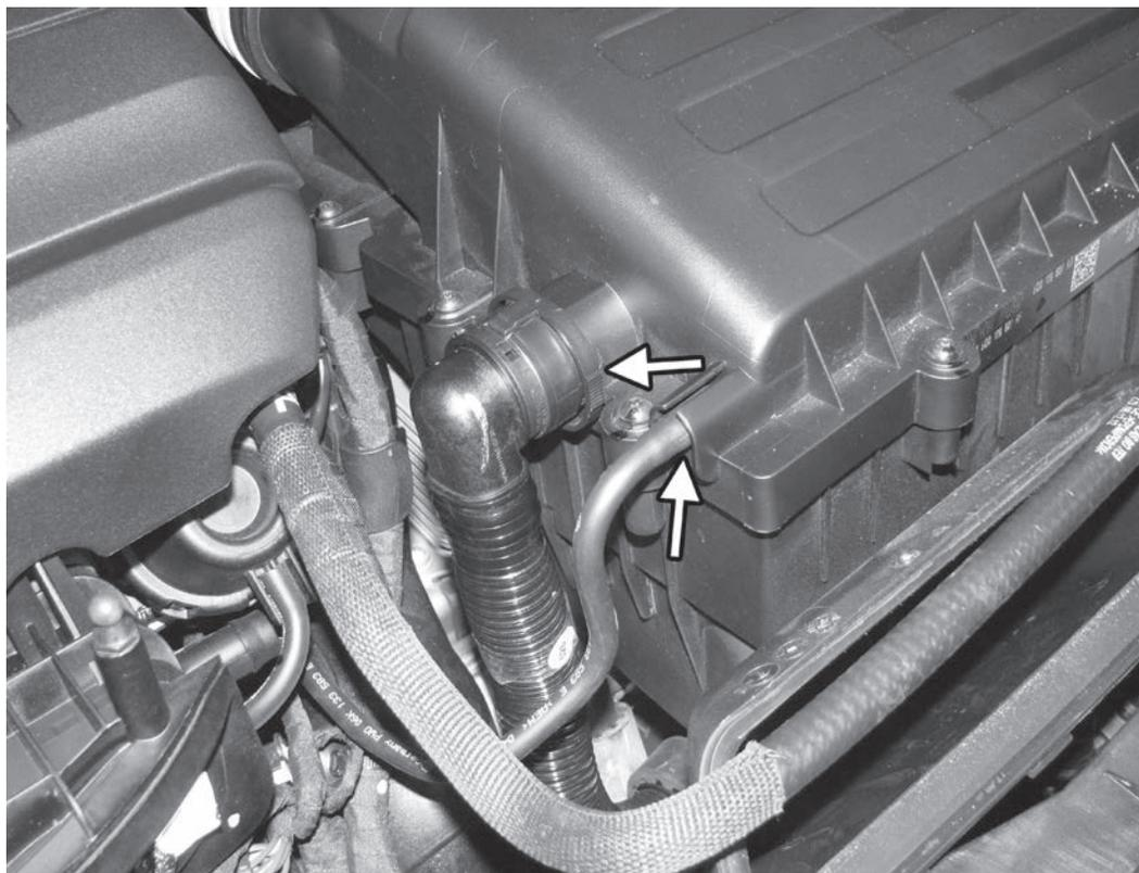
7) Remove the vacuum line from the front right corner of the factory airbox by pulling it off. Then, if equipped, remove the connection to the secondary air pipe by pressing down on both sides of the fitting and pulling away from the airbox.
