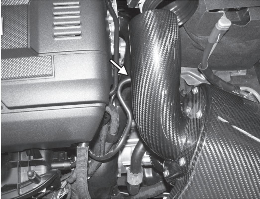
15) Connect the vacuum line that was on the right side of the factory airbox to the vacuum port on the bottom of the APR intake tube.
