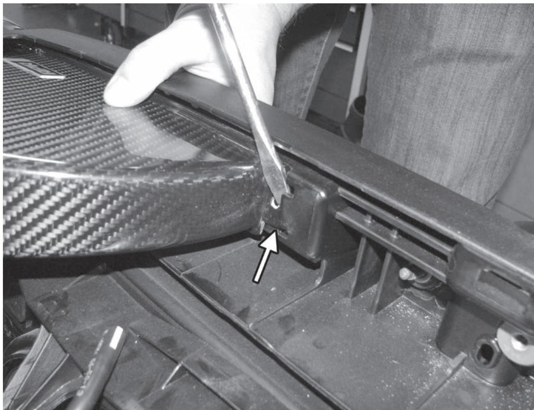
13) Loosely place the APR intake in the car. Slide the right mounting tab of the intake underneath the mounting point on the back of the factory radiator support. It may be necessary to carefully pry the factory tab back for the APR intake to fit. Once in place, slide the entire APR intake to the right side of the car to lock it in place.
