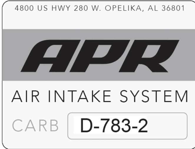
17) Once the APR intake is installed, be sure to clean a visible location under the hood and affix the supplied sticker in order to aid inspection of the vehicle under the California Smog Check program.
